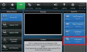
Some systems have a separate control controls for the audio on the 'Send to' tab. This gives the user the ability to see this audio routing concept a bit easier.
